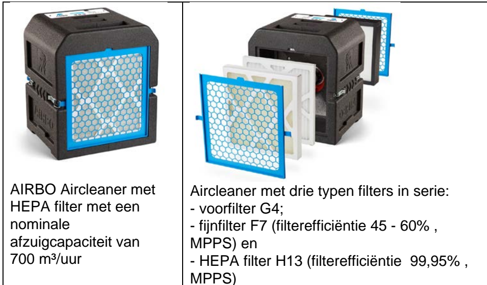
Figuur 1. AIRBO Aircleaner
